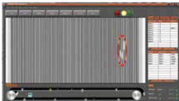
Report showing steel cord damage.
