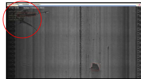
Image of damage to edge of belt
